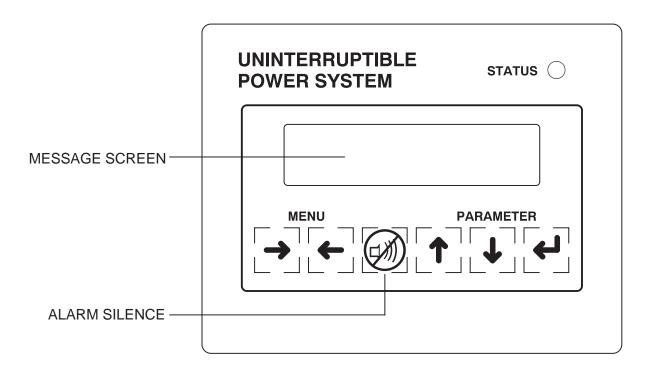
Figure 3–1. Digital Monitoring Panel
