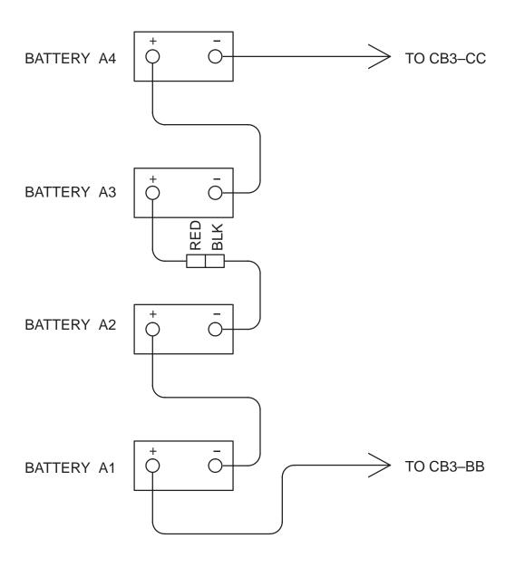
Figure 2–2. Battery Interconnection Diagram
